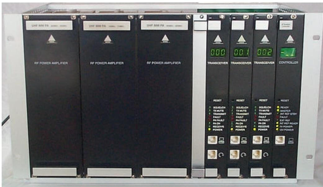
Users of Westel’s existing DRB-25 product may upgrade to the *Trunkissimo* platform re-using their existing Controller, Transceiver and Power Amplifier modules. *Trunkissimo* may also be used in a P25 conventional (non-trunked) mode and may be stacked for a total of 6 channels.
